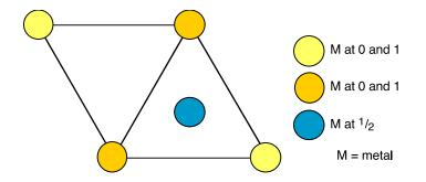
The vertex atoms are shared between 8 unit cells, but do not contribute equally to all of them. Those shown in orange in the cell projection diagram contribute  $\frac{1}{6}$  to the unit cell, whereas those shown in yellow contribute only  $\frac{1}{12}$ . The atom in blue is fully within the unit cell. This means there are  $(\frac{1}{6} \stackrel{\checkmark}{} 4) + (\frac{1}{12} \stackrel{\checkmark}{} 4) + (1 \stackrel{\checkmark}{} 1) = 2$  atoms in the unit cell.
