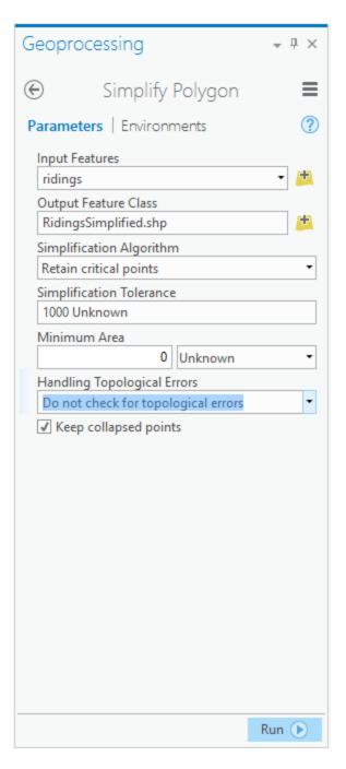
There are two choices for simplification. The first, retain critical points, eliminates unneeded points while preserving the shape of the polygon. Retain Critical Bends
