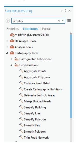
Now, click on Simplify Polygon. This will bring up the simplify polygon pane. Choose the shapefile or geodatabase feature class to be simplified from the dropdown list under Input Features. In Output Feature Class, enter the name of the new simplified shapefile or feature class. Clicking on the folder + icon allows you to change save location from the default geodatabase for the project.
