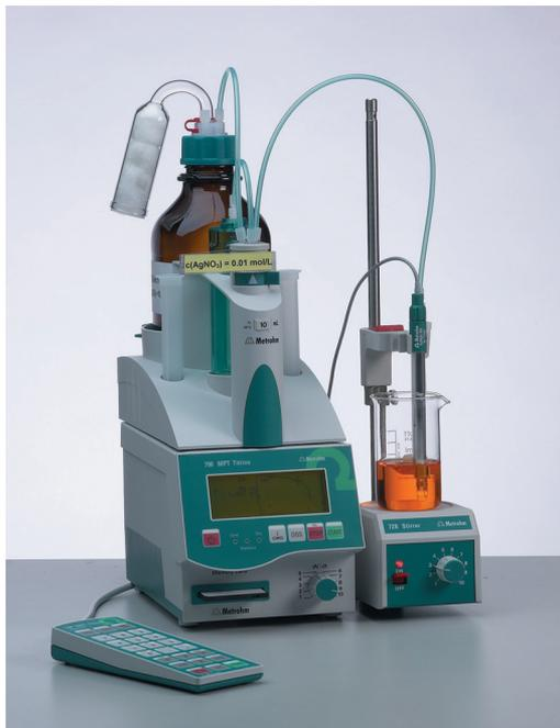
**Figure 1.11** Automated titration apparatus used to carry out routine acid-base titrations in industry.
