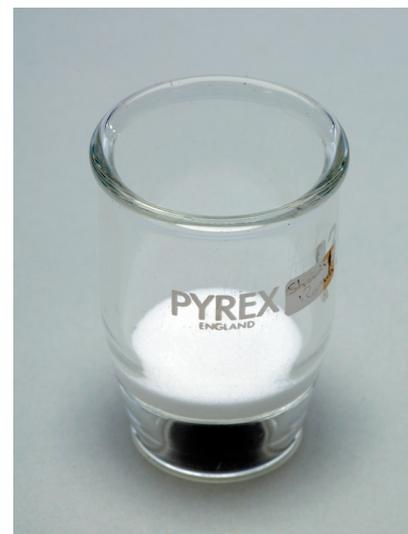
**Figure 1.12** A sintered glass weighing crucible.
