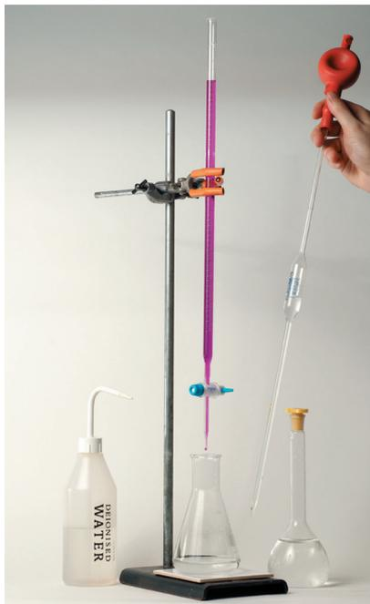
**Figure 1.10** Typical apparatus for a titration, showing a burette, pipette, and a volumetric flask used for making up a standard solution.
