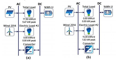
**Figure 2.** (a) Schematic Diagram of HOMER Simulation for Full House Load (b) Schematic Diagram of HOMER Simulation for Only Electrical Load
