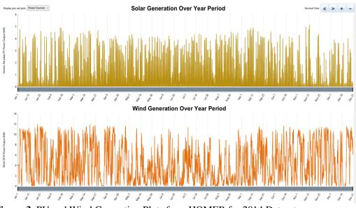
Figure 3. PV and Wind Generation Plots from HOMER for 2014 Dataset
