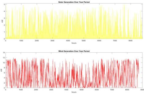
Figure 4. PV and Wind Generation Plots from MATLAB for 2014 Dataset
