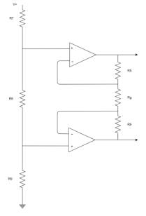
Figure 4: First stage of instrumentation amplifier
