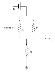
Figure 1: Thermistor linearization circuit set up on a bread board to measure the voltage for different temperatures and values of R1 and R2.
