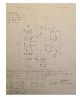
Figure 7: Thermocouple circuit with nodes labeled for prototyping board
