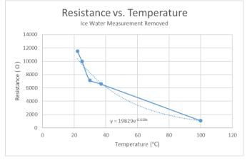
Figure 9:Resistance vs. temperature curve plotted from Table 1 with 0°C measurement removed
