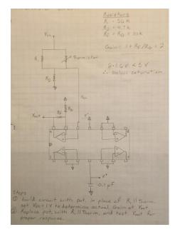
Figure 3: Thermistor linearization circuit with amplifier
