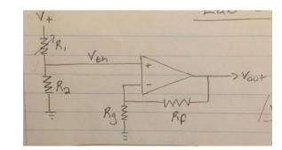
Figure 2: Operational Amplifier, non-inverting gain circuit
