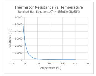
Figure 10: Best fit line for the thermistor used in this lab, based on the Steinhart Hart equation
