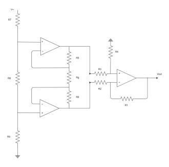
Figure 5: Instrumentation amplifier, stage one and two
