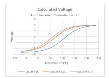
Figure 12: Voltage curves calculated using Equation 9
