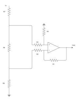
Figure 6: Second stage of instrumentation amplifier connected to voltage divider
