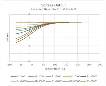
Figure 14: Voltage curves calculated using for a fixed value of R2 using Equation 9
