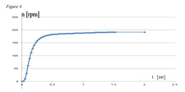
Figure 4 shows the rotation speed of an inverter motor when 34.4 Newton meters are applied.Y axis shows rotation speed in revolutions per minute, and the x axis shows time (Bitar, 2012). The steep acceleration curve shows that the rpms level out consistently, giving the motor a steady rotation speed.
