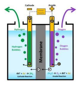
$\begin{array}{c} 2H_20+2e^- \rightarrow H_2+2OH^-\\ 2OH^- \rightarrow H_2O+\frac{1}{2}O_2+2e^-\\ (\text{U.S Department of Energy, 2018}) \end{array}$
