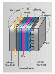
Cathode:  $O_2 + 4H^+ + 4e^- \rightarrow 2H_2O$ Anode:  $2H_2 \rightarrow 4H^+ + 4e^-$ Net:  $2H_2 + O_2 \rightarrow 2H_2O$ (Hydrogenics Fuel Cell, 2018)
