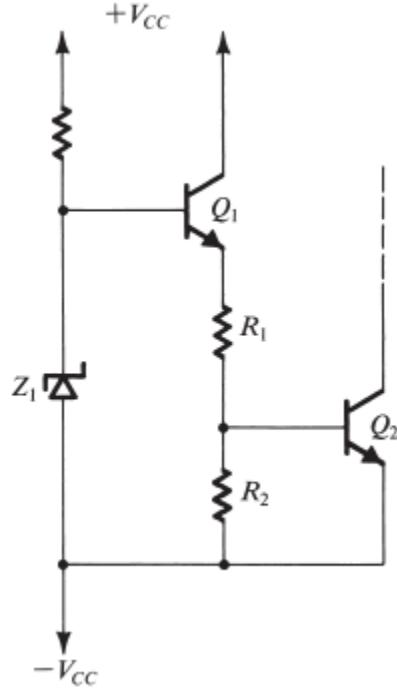
Figure x4.4 Thermal-shutdown circuit.
