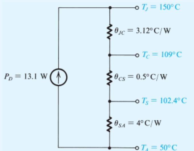
Figure x4.10 Thermal equivalent circuit for Example x4.2
