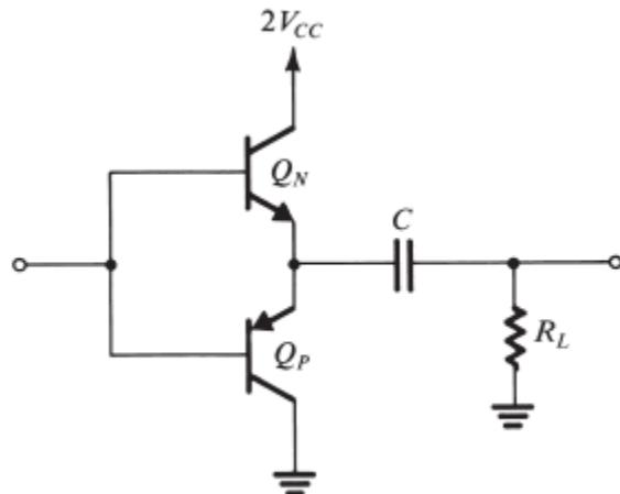
**Figure x4.2** Class B output stage operated with a single power supply.
