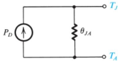
Figure x4.6 Electrical equivalent circuit of the thermal conduction process;  $T_J - T_A = P_D \theta_{JA}$ .
