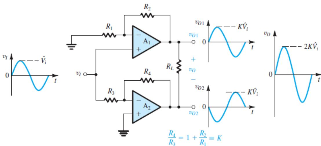
Figure x4.14 The bridge amplifier configuration.
