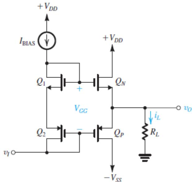
**Figure x4.5** Classical CMOS class AB output stage. This circuit is the CMOS counterpart of the BJT circuit in Fig. 12.13 with the biasing diodes implemented with diode-connected MOSFETs  $Q_1$  and  $Q_2$
