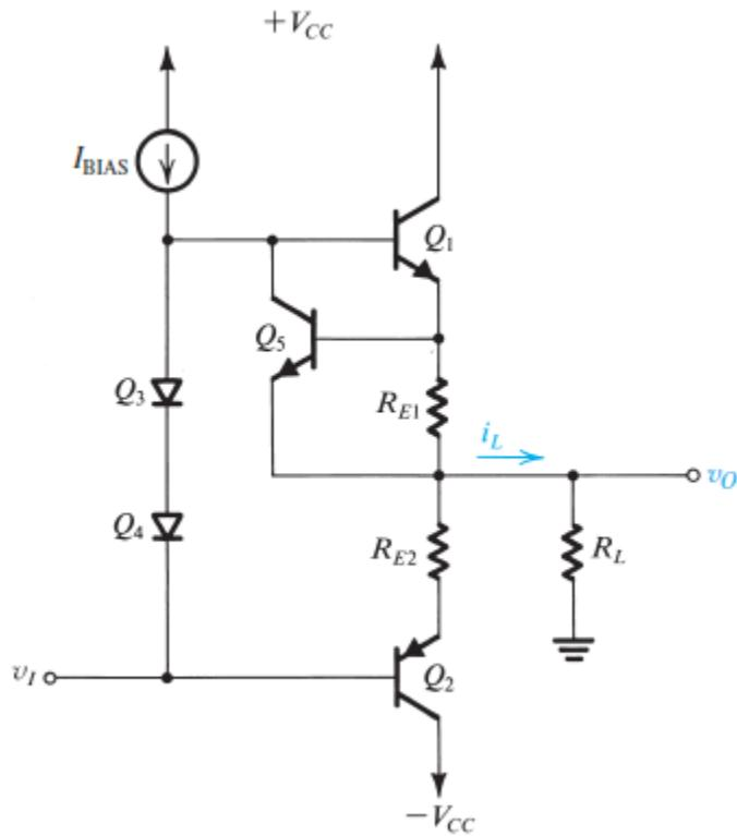
**Figure x4.3** A class AB output stage with short-circuit protection. The protection circuit shown operates in the event of an output short circuit while  $v_o$  is positive.
