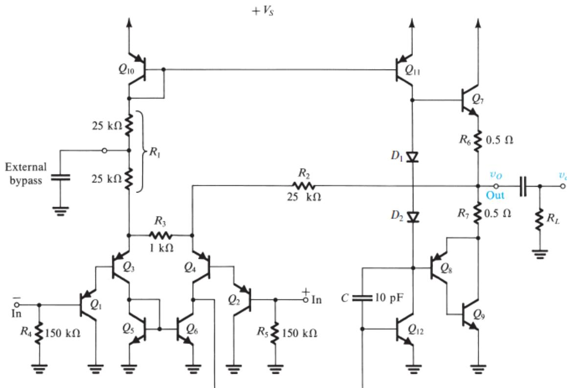
**Figure x4.11** The simplified internal circuit of the LM380 IC power amplifier. (Courtesy National Semiconductor Corporation.)
