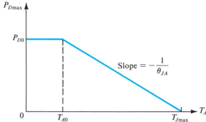
**Figure x4.7** Maximum allowable power dissipation versus ambient temperature for a BJT operated in free air. This is known as a “power-derating” curve.
