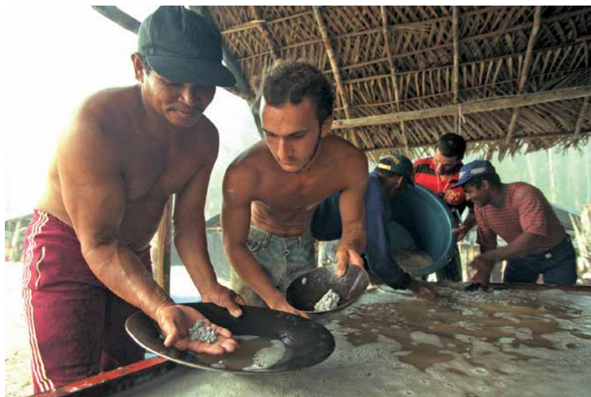
Figure 1 Amalgamation Often the gold is so small that it is not easily seen or removed by panning methods—a lot can just float away. Mercury captures the gold in an amalgam. Gold miners crush rock that contains gold; extract as much rock by washing it away, or if the gold is in mud, just wash away the mud and let the gold settle out or float in the water; combine the remains (gold dust or bits) with mercury to form a ball (combined mercury and gold), as shown in the figure; and then burn off the mercury leaving the gold behind.
